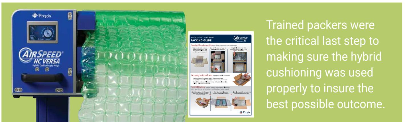
In this instance, an 18-inch wide pad with large (1 ¼-inch) cell height met the project goal of reducing damaged product incidents.
