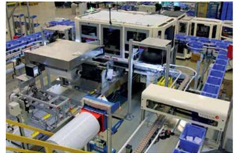
The Sharp MAX™ Proline Bagger with a custom dual-stage funnel allows this manufacturer to count / accumulate product and then seal the bag in one continuous process. As the product stream continues uninterrupted, the entire line keeps running even as the bag is sealed.
