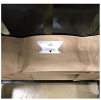
Cut the sleeves inward with a strap cutter, pull the sleeves straight out holding the bundle with your other hand.
