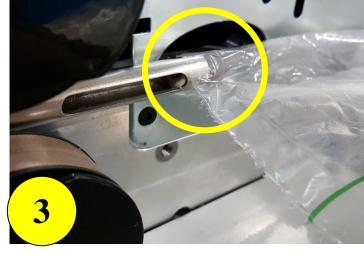
3. Thread Film Opening onto the Tube.
