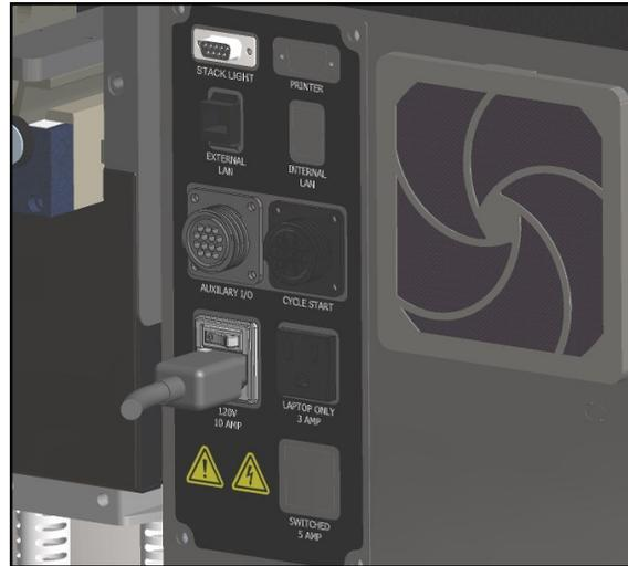
**Figure 2-1A. Electrical Connections.\***
