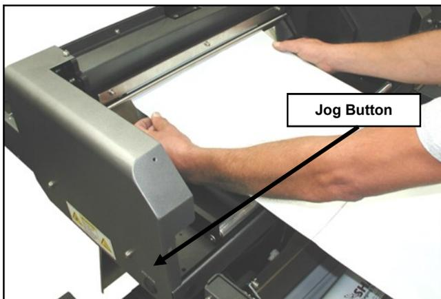
**Figure 2-5A. Web centered on Drive Roller.**
