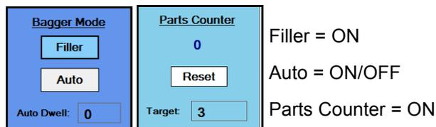
**Actual Count** – The number below “Parts Counter” displays how many parts have been counted. This number resets to 0 once the bagger cycle is initiated or if Part Counter is turned off. The Target is determined in the Job that has been loaded from Job Setting Screen.
