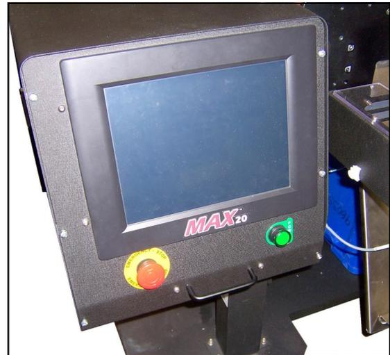
**Figure 5-1A. E-Stop & Power Pushbutton.**
