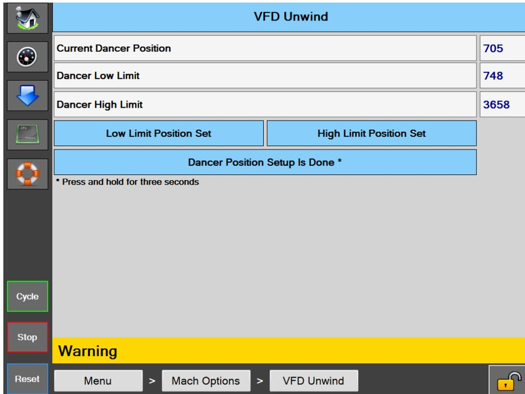
**Figure 4-25A. VFD Unwind Screen**
