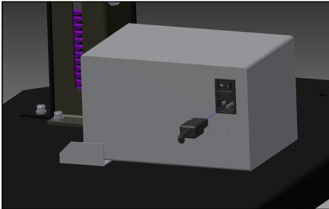
2. Turn switch to the ON position. The HMI will automatically start up when Power Entry Module Switch is turned ON.
