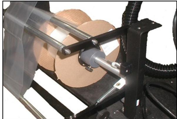
**Figure 2-3B. Core Chuck & Unwind Shaft.**
