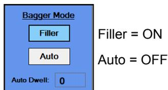
With Filler ON and Auto OFF, the bagger will run in "Filler Mode". This mode cycles a single bag out each time and requires the operator to initiate a Cycle Start for each bag. In this mode, a filler device or machine does the actual loading or filling of the open bag.
