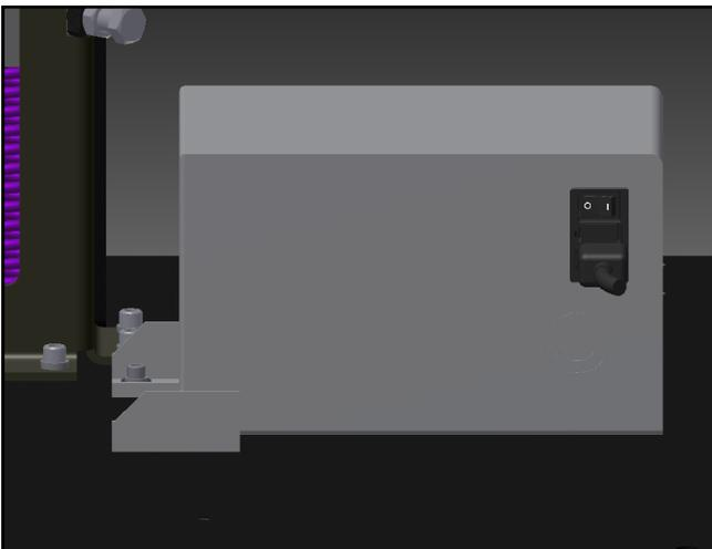
3. Release the E-Stop Button and press the Green Power Button. The green light should illuminate and energize the MCR.
