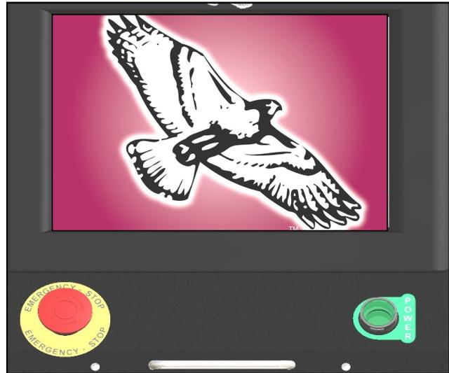
**Note:** If the bagger has the Stack Light option, the horn will sound until the HMI program has finished loading. To prevent horn blowing, do not press the Green Power Button until HMI program is loaded. The horn then can be silenced by pressing the Reset Button.
