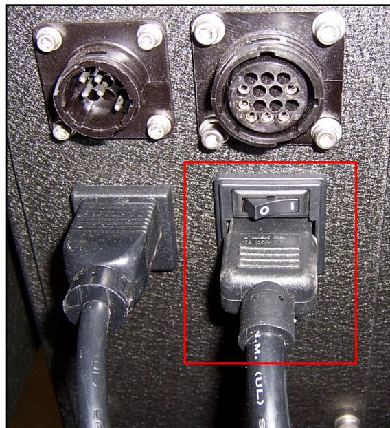
**Figure 5-1B. Power Entry Module Switch.**
