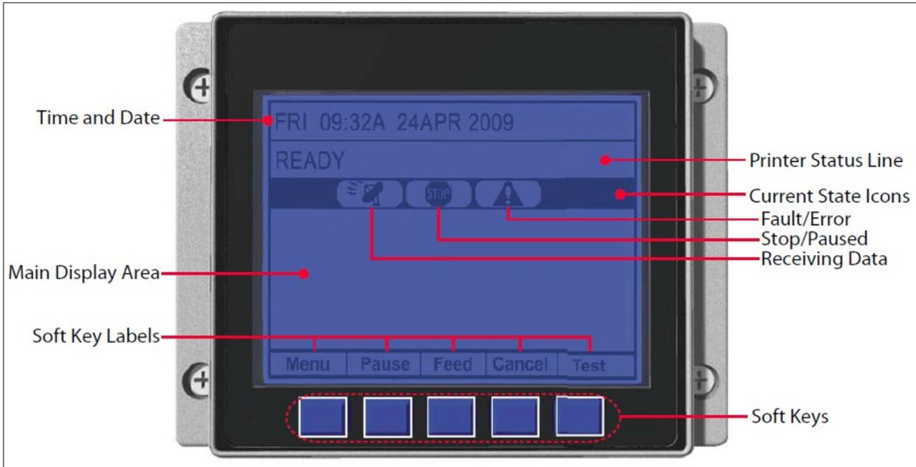
The graphic display is a window into printer operations, displaying the following information
