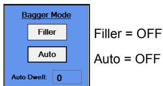
Both the Filler and Auto buttons are OFF at the HMI. In manual mode the operator hand loads or fills each opened bag and then cycles the bagger. The operator initiates a cycle by one of these methods:
