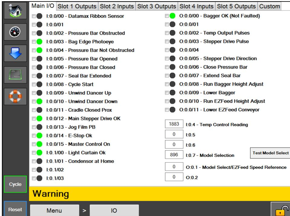
Figure 4-3A. Input/output Screen.
