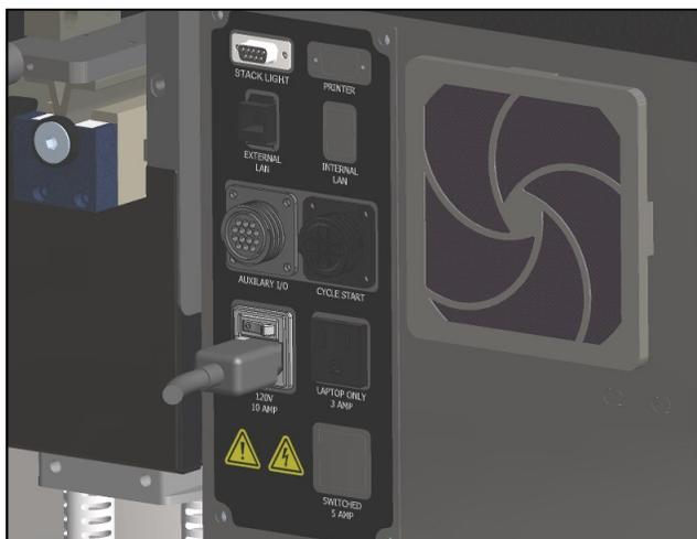
2. Turn switch to the ON position. The HMI will automatically start up when Power Entry Module Switch is turned ON.
