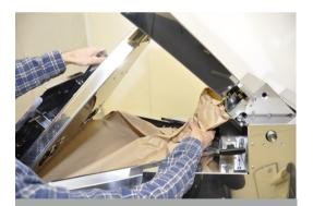
Cut the paper across the rods with a knife, at the infeed guide rods.
