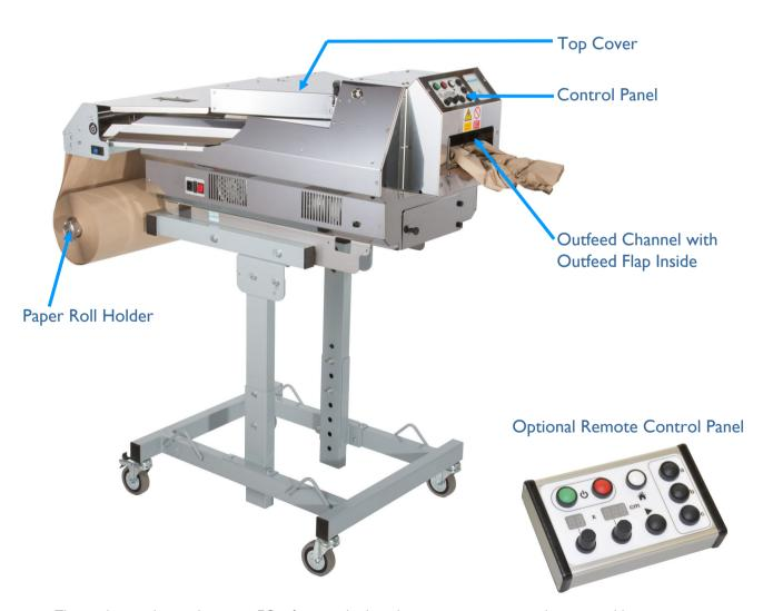
The machine is designed to meet EC safety standards and requires connection only to a suitable electrical supply. Noise levels not to exceed 70dB(A).
