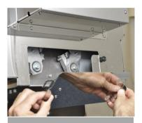
The machine will not switch on, or run with the paper off-cuts door open.
