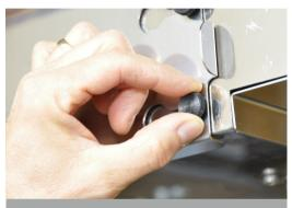
Slacken the two black knobs securing the paper off-cuts door under the
