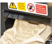
The machine will not switch on or start if the outfeed flap is open.
