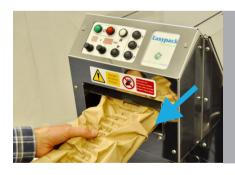
1. Remove any material from the outfeed channel and ensure the outfeed flap is closed.
