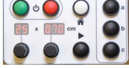
2. Rotate the length knob to the required pack length.
