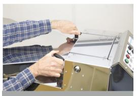
Unscrew the two black 'T' handles each side of the top cover until they swing down
