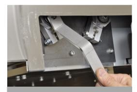
**4.** Locate the blade reset tool (supplied) on the crank nut.
