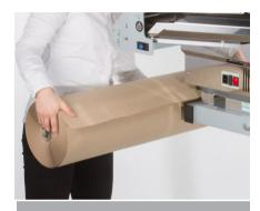
Noting the unwind direction, slide a new roll of paper onto the paper arm until the sprung retaining latch springs up.
