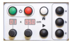
Release the preset button to save the values - the display will flash twice before remaining on.
