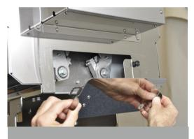
Lift the door forwards over the knobs to remove.
