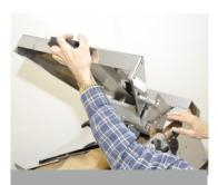
The machine will not switch on, or run with the top cover lifted up.
