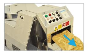
**4**. Remove the material from the outfeed channel and the machine will generate
