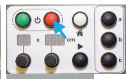
5. The machine can be stopped by pressing the red "O" button.
