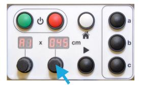
2. Rotate the length knob to the required pack length.
