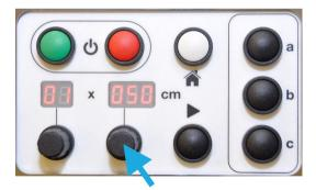
3. Rotate the length knob to the desired length (whilst the display is flashing).
