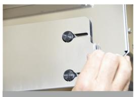
2. Slide the door to the right to release the key tongue from the safety switch.
