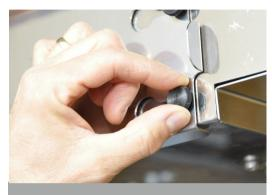
I. Slacken the two black knobs securing the paper off-cuts door under the outfeed channel.
