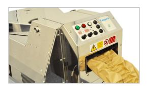
3. The machine will produce the preset quantity and length of packs to the set length.
