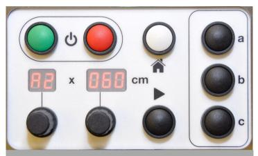
The machine will only operate when the display is illuminated
