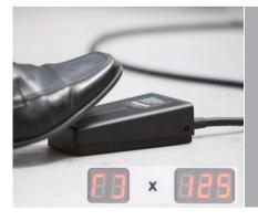
2. Depress and hold down the footswitch. The length display will increment up as the pack is produced and the quantity display will change to a cycling symbol.
