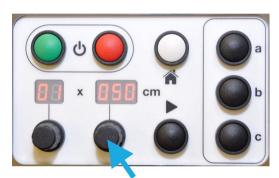
**2**. Rotate the length knob to the required length.
