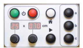
3. Remove any material from the outfeed channel. Check there is ample space for the packs to discharge from the 'Start' button to initiate the cycle.
