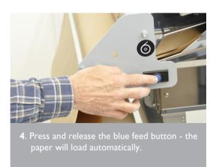
The quantity display will flash 'Ld' whilst the paper is loading. Once loading is complete the display will revert to the previous settings.
