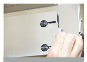
2. Remove the paper off-cuts door by sliding to the right and lifting forwards.
